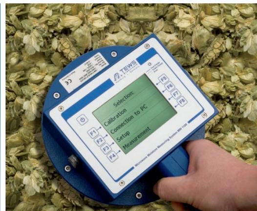
**Measuring range** The actual measuring range is specific to the material under analysis and can be selected in some sections. Supported product temperatures range from 5°C to 60°C, are read using the integral infrared temperature sensor and are compensated by optional thermally stabilized calibration.
