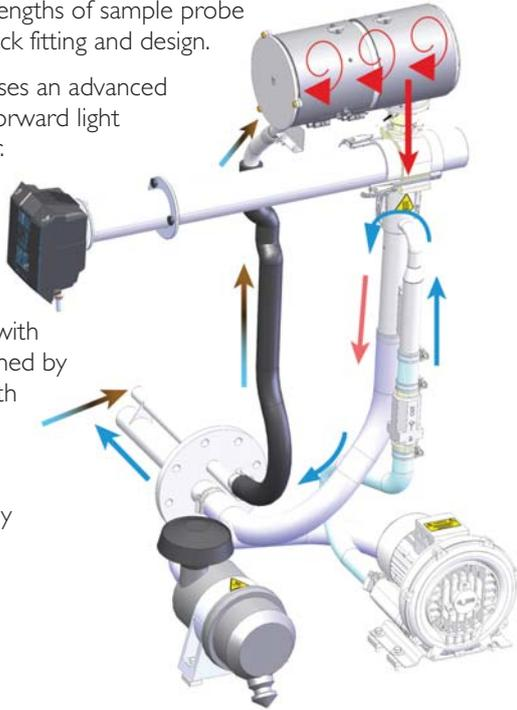
The QAL 182 WS utilises direct extractive heated sampling which can be configured to either extract an isokinetic sample or extract a sample based on a pre-set user-defined velocity. The extracted sample passes directly into a heated vaporising chamber. The sample is superheated and exits into a controlled sample chamber. The ProScatter® sensor provides a high accuracy, high resolution measurement meeting ELV's of 15mg/m<sup>3</sup> or less.
