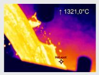
Measurement of a pouring stream
