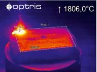
Measurement during laser welding process
