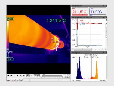
The software can be used to save the recording from the thermal imaging camera as video sequences which can then be saved for analysis later on. The video sequence is recorded for every pixel including all temperature information. An integrated screen capture function makes it simple to retrospectively generate videos in wmv format.
