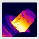
In drop forging, the semi-finished products must be at a certain forging temperature before forming. In order to achieve the optimum production result, the surface temperature of the material is controlled ccordingly.
