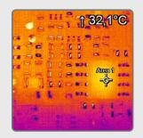
More and more manufacturers of electronic circuit boards rely on non-contact temperature measurement due to the constantly increasing performance of their components.
