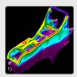
In order to prevent component distortion during injection molding, the process is monitored by thermal imaging cameras detecting and adjusting temperature overor undershoots during molded part measurement.
