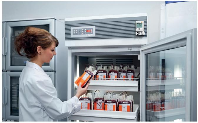
A WiFi data logger monitors the temperature in a blood refrigerator, and provides the staff with an alarm when critical deviations occur.
