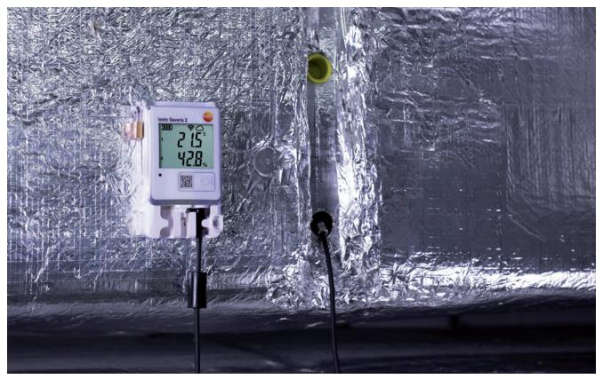
A testo Saveris 2 WiFi probe measures temperature and humidity in a ventilation duct.
