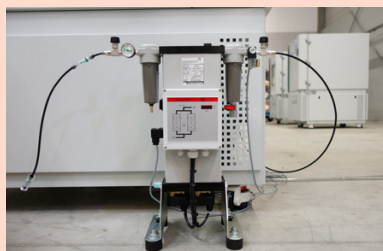
Compressed Air Dryer
