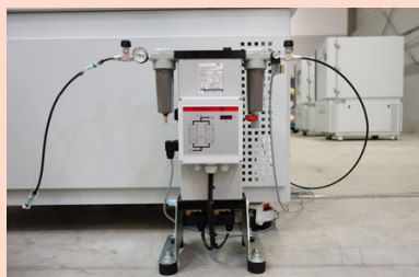
Compressed Air Dryer
