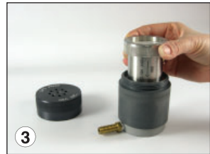
Insert media cartridge into cartridge holder section.
