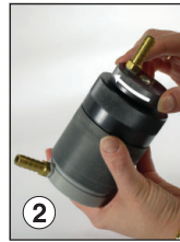
Thread calibration adapter into sampling head inlet.
