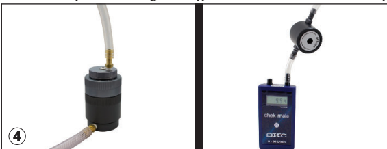
Unscrew quick-connect plug on side of case. Use tubing with quick-connect fitting to attach case (pump) inlet to exhaust of sampling head.
