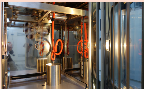
Cold Bend Cables Testing
