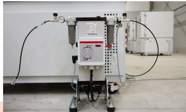
Compressed Air Dryer
