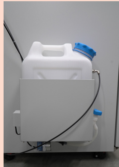
Water supply tank
