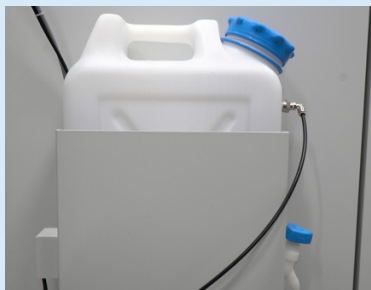
External Water tank
